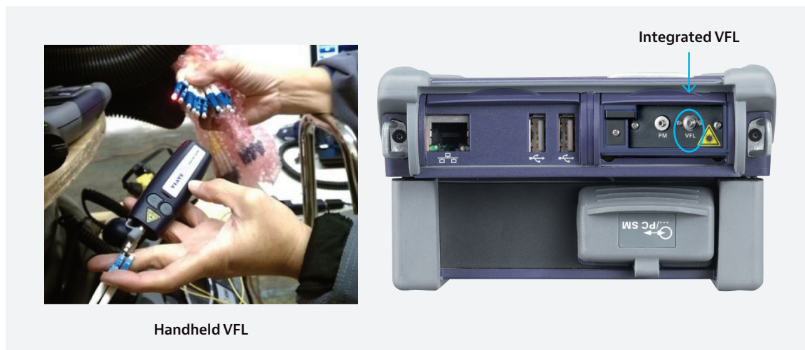
Figure 2: Fiber continuity test
