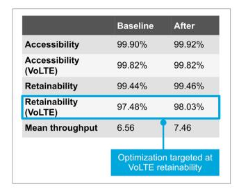
Automated optimization used subscriber-centric intelligence to analyze the current subscriber usage. Based on this intelligence, power changes were made to 67 cells, and 63 cells received antenna e-tilt changes. The result was a 1.3-point improvement in the LTE quality index and a 24 percent increase in data traffic volume – all without affecting 3G voice services. See diagram on left of page.
