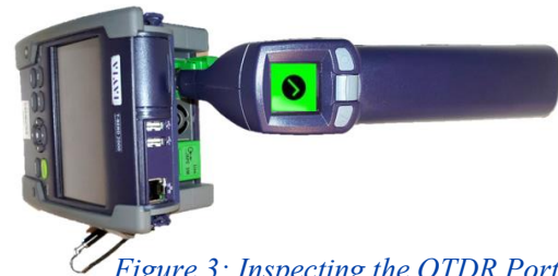
Figure 3: Inspecting the OTDR Port
