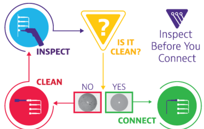
Figure 2: Inspect Before You Connect
