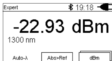
Fig. 3 Display in Auto- \lambda mode showing one detected wavelength and the power level.
