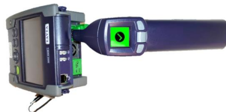
Figure 5: OTDR Port Inspection
