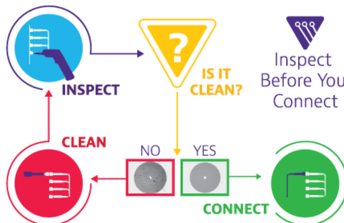
Figure 11: Inspect Before You Connect
