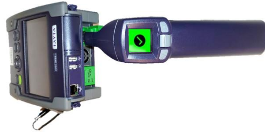
Figure 3: OTDR Port Inspection
