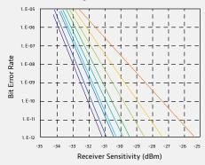
BER measured as a function of power delivered to the RX
