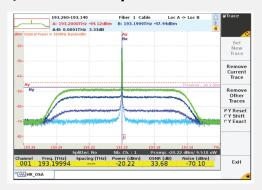
Varying power levels of OSNR inside a DWDM channel
