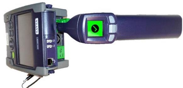
Figure 3: OTDR Port Inspection
