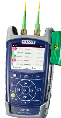
OLP-87 G & XGS-PON or NG-PON2 Selective PON power meter
